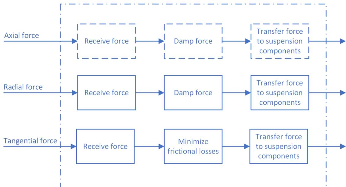
**Figure 15.** *Function structure of a guide shoe contacting element*
