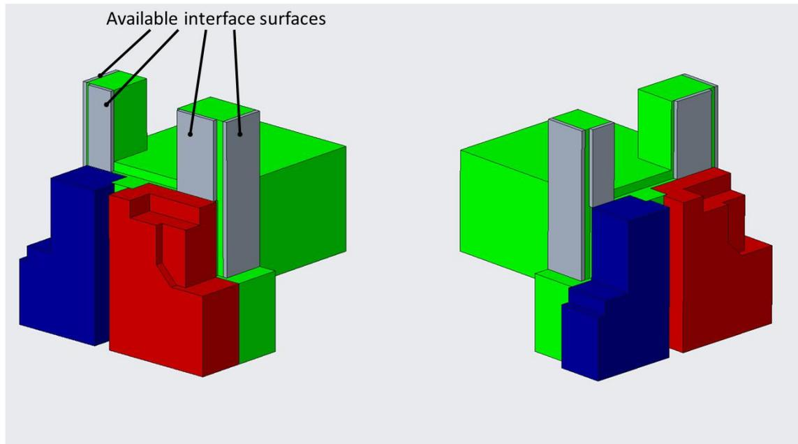
**Figure 13.** Available space with available sling interface surfaces
