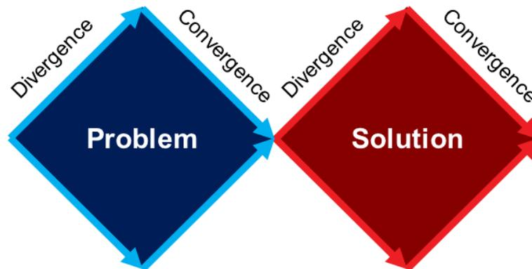
**Figure 7.** *The double diamond design process model [22]*
