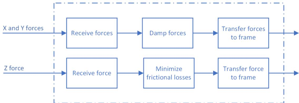
**Figure 14.** *Function structure of a guide shoe*
