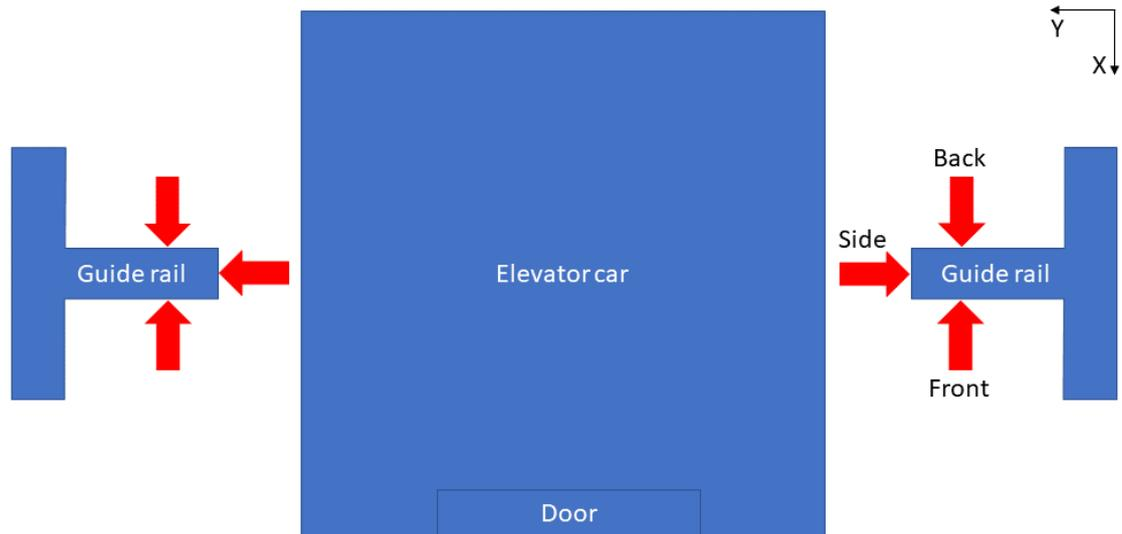
**Figure 4.** Directions of restriction. NOTE: not in scale
