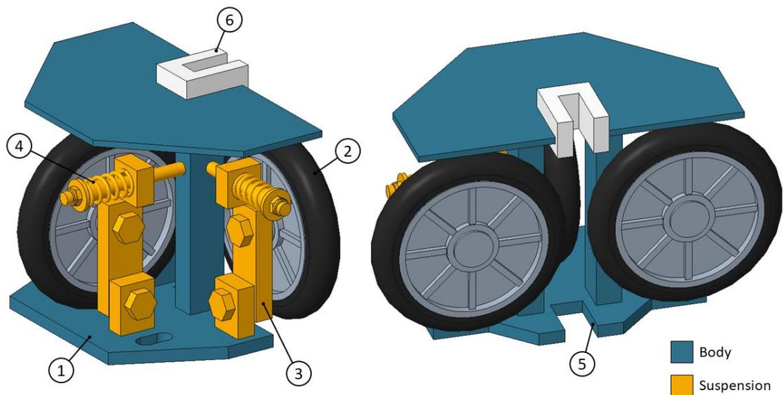
**Figure 2.** Model of a traditional type of spring suspended roller guide. Components as numbered: 1 – body, 2 – roller, 3 – lever arm, 4 – spring system, 5 – safety throat, 6 – removable slider
