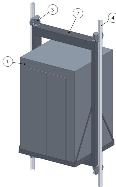
**Figure 1.** A visualization of the main components of elevator guiding system with a car enclosure. Components as numbered: 1 – car enclosure, 2 – sling, 3 – guide shoe, 4 – guide rail
