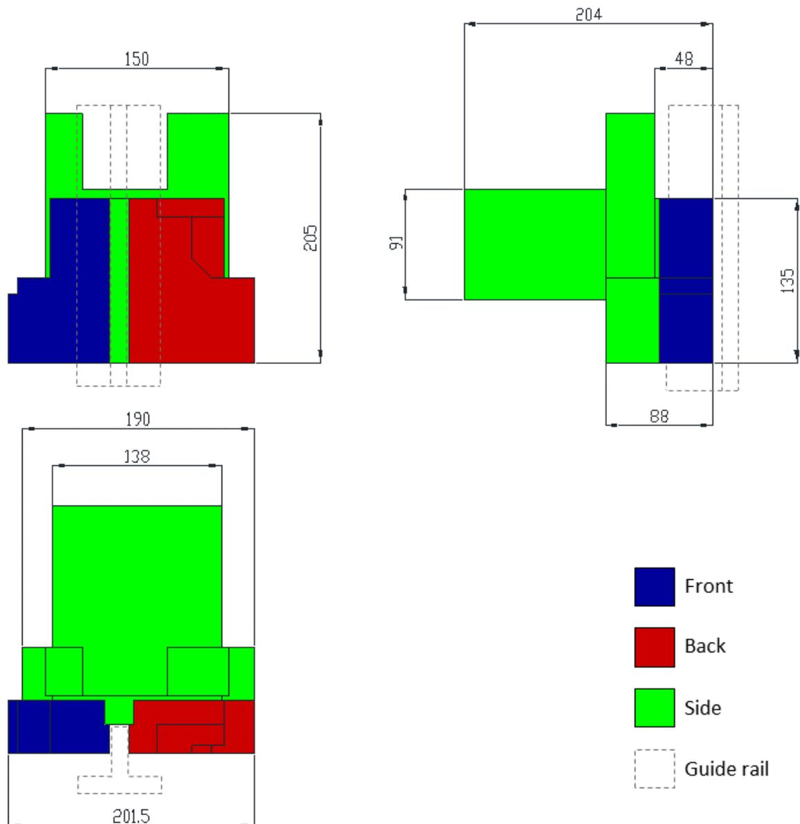
**Figure 12.** Space available for roller guide with some main dimensions
