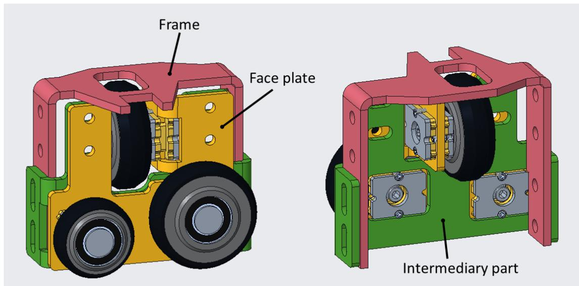
**Figure 19.** *Variant E3\_1 body parts named*
