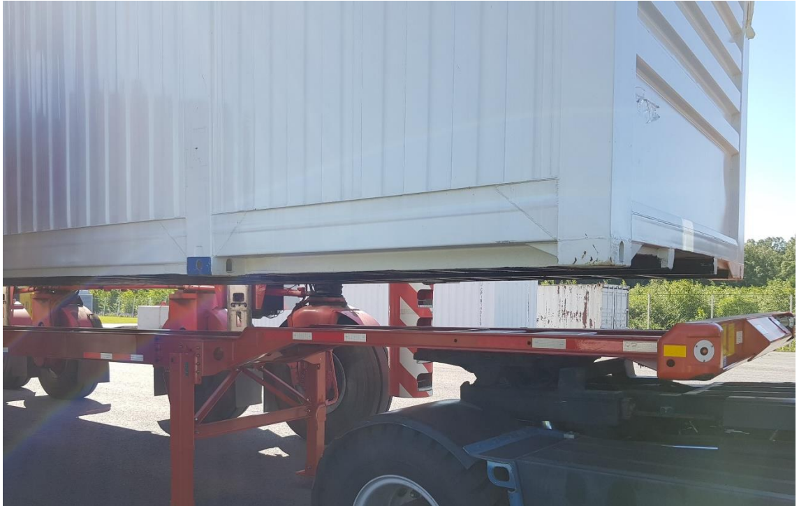
Figure 4.2 Scene of container placing on truck chassis with a gooseneck
