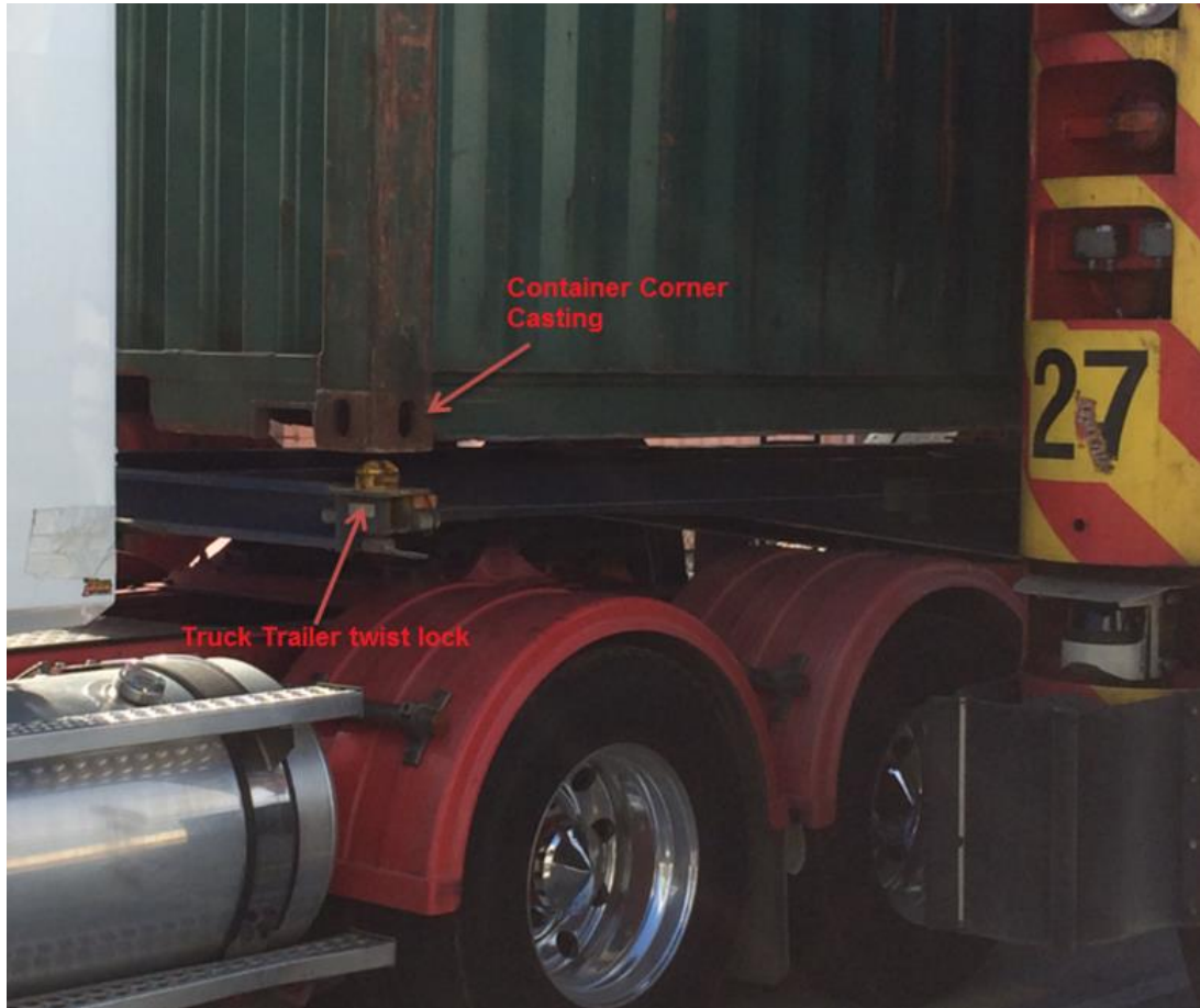
Figure 4.1 Scene of container placing on truck chassis with twist locks
