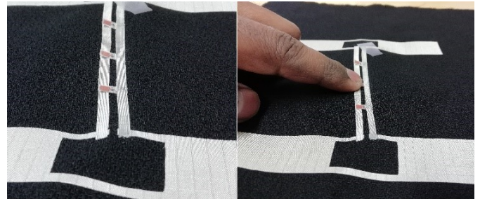
Fig. 4. All IC copper pads are initially separated from the antennas (left) and a specific IC can be “activated” by touching the copper pad, which will connect the IC to the antennas (right).
