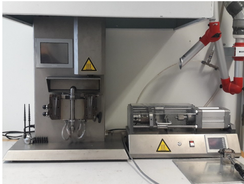
Figure 24. The micro compounder (left) and the micro injection moulding machine (right) from Xplore Instruments.
