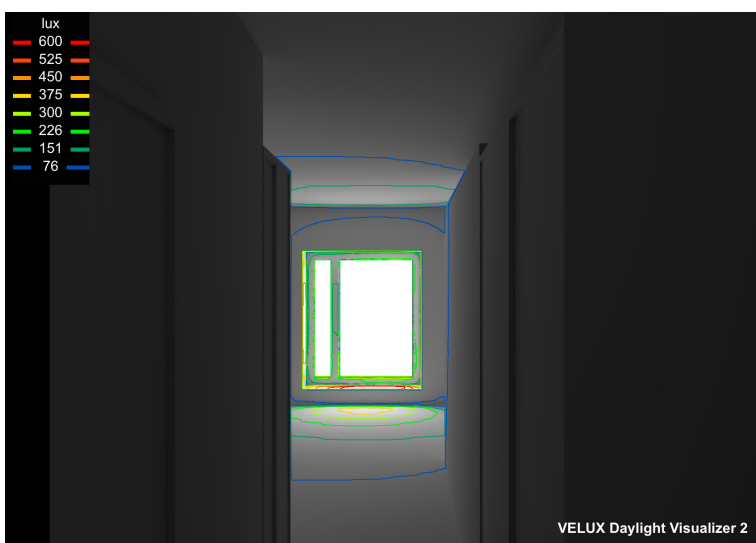
Figure 8 Illustration of illuminance of apartment 1-A during March at 12:00, with overcast sky.
