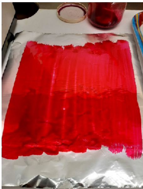
Figure 1. Pinhole test for SAGA aluminium foil and no pinholes were detected.
