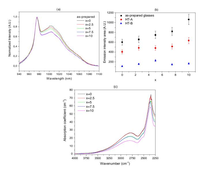
**Figure 3:** Emission spectra measured using a 900 nm excitation (a), integrated area of the emission band (b) and IR absorption spectra of the glasses (c)
