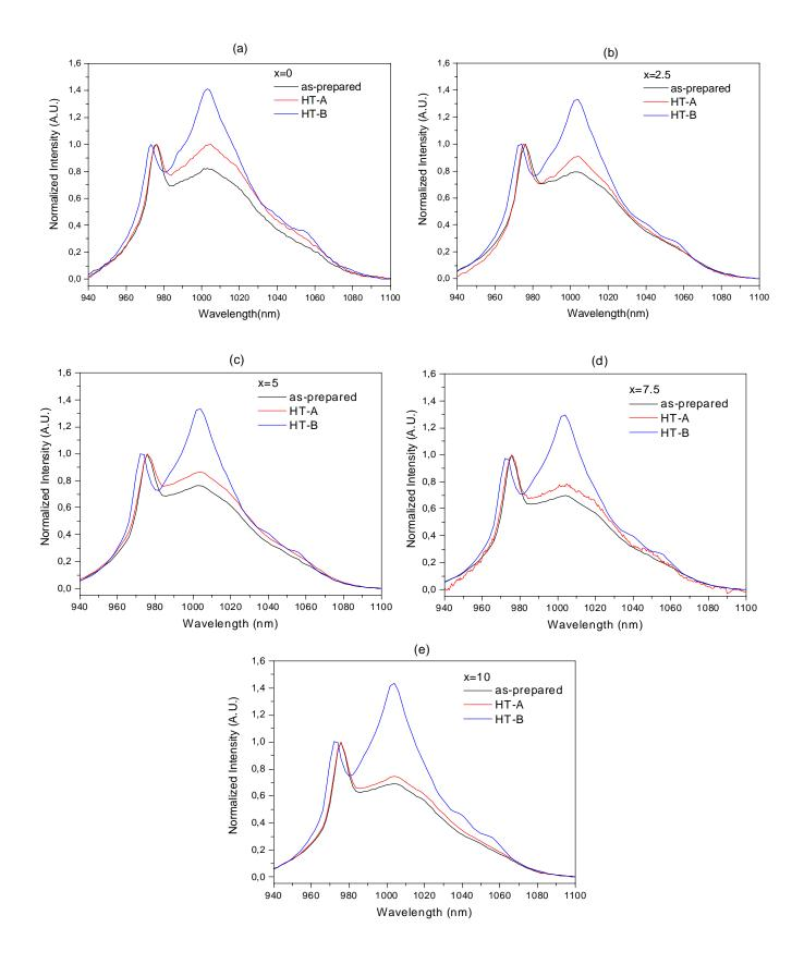
**Figure 6:** Normalized emission spectra of the glasses with (a) x = 0, (b) x = 2.5, (c) x = 5, (d) x = 7.5 and (d) x = 10 prior to and after heat treatment A or B. Excited at 900 nm.
