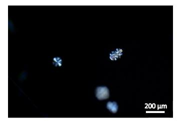
**Figure 9:** Optical images of the crystals found in the heat treated glasses with x = 0 after HT-A (a), HT-C (b) and HT-D (c). The images were taken with 5x microscope magnification in transmission mode using cross-polarized configuration of the microscope
