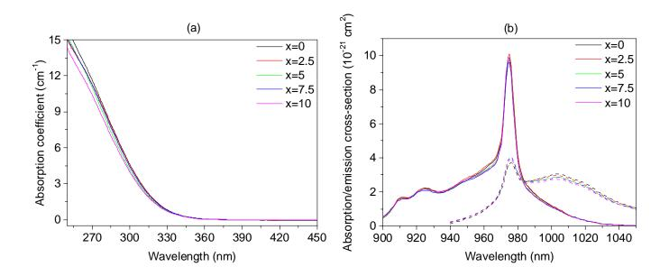
Figure 2: Absorption spectra (a) and absorption/emission (solid/dashed) cross sections centered at 975 nm (b) of the investigated glasses.
