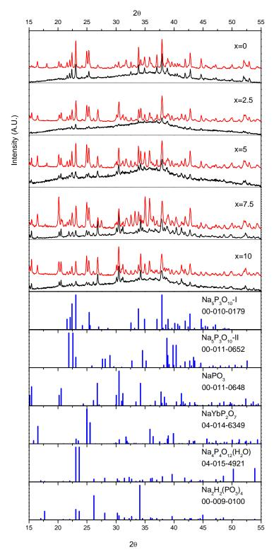
Figure 5: XRD of the investigated glasses after heat treatment A (black), and B (red)
