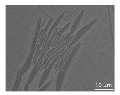
**Figure 7:** SEM image of crystals found in the volume of the glass with x = 0 after heat treatment A
