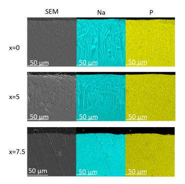
Figure 4: Elemental mapping of the crystals in the glasses' SEM images after heat treatment A
