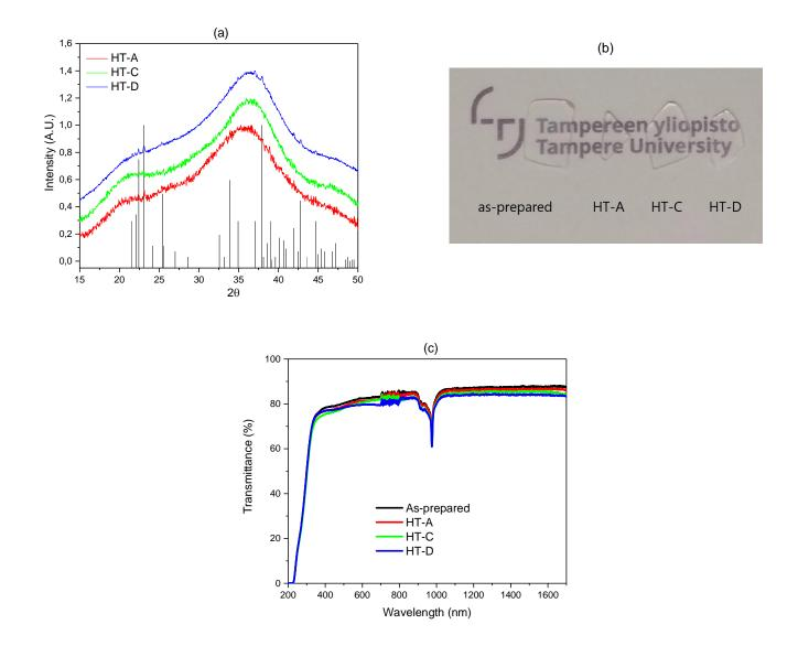
**Figure 8:** XRD patterns (also shown is the XRD pattern of Na<sub>5</sub>P<sub>3</sub>O<sub>10</sub>-I [00-010-0179]) (a), the pictures (b) and the transmittance spectra (c) of heat treated glasses with x = 0
