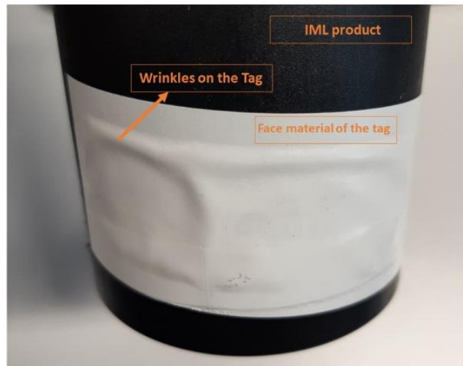
Figure 2. Wrinkled RFID tag after IML process.
