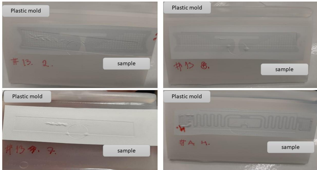
Figure 38. Case 1 contains samples with mesh designs with wrinkles.
