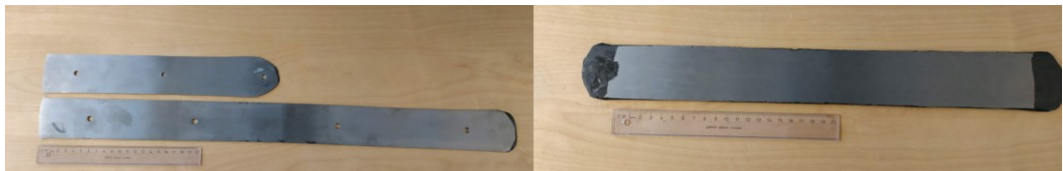
Figure 7.1 Cantor (left) and \text{Al}_{0.3}\text{FeCoCrNi} (right) plates.
