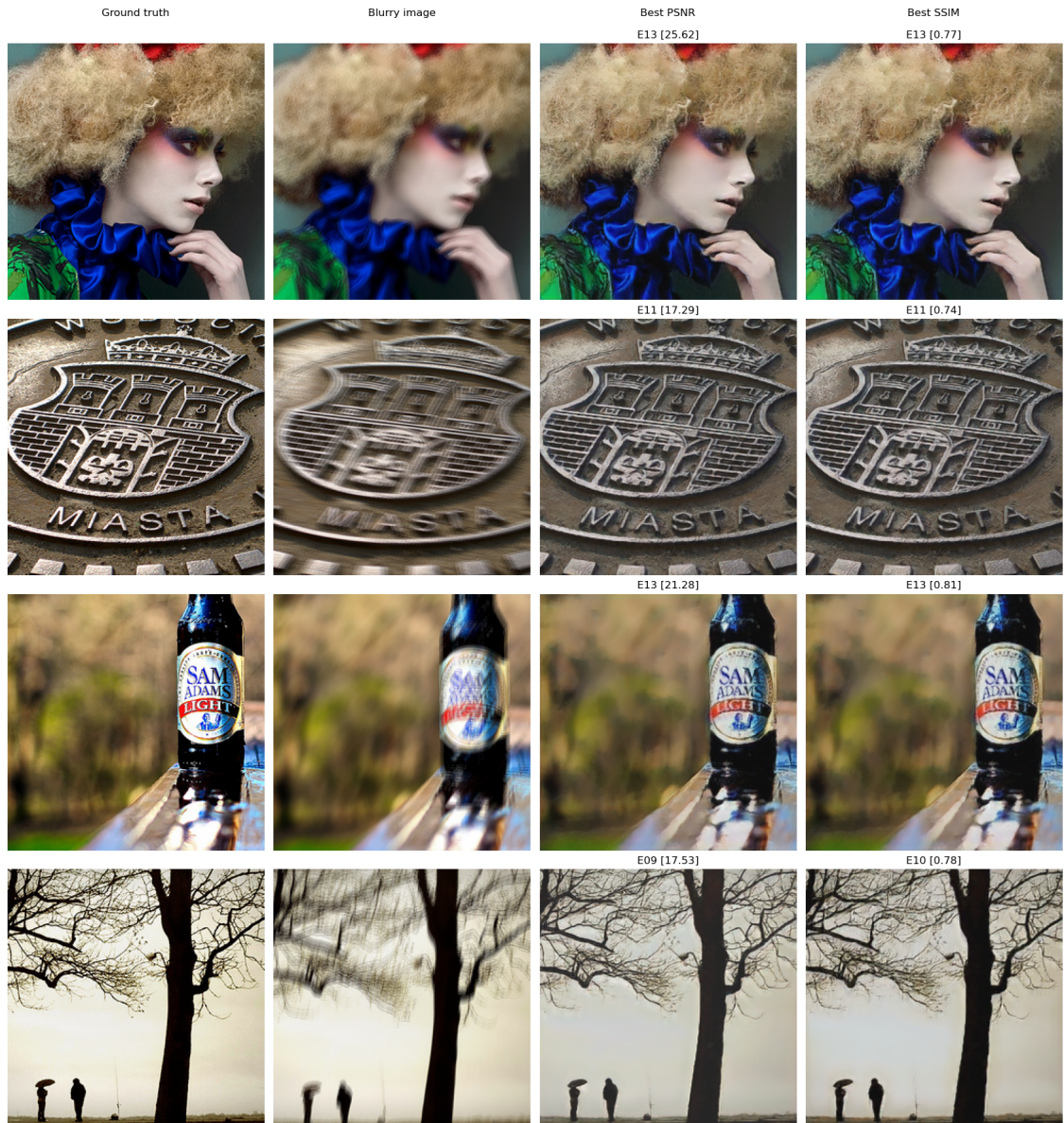
Figure 3.8. De-blurred images from testing data, picking best by PSNR and SSIM among all models developed.
