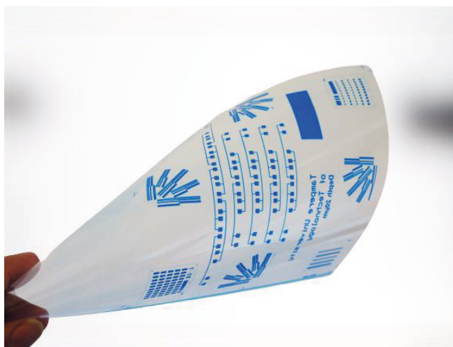
Figure 1. The array of electronic pattern on flexible substrate (for illustrative purpose).
