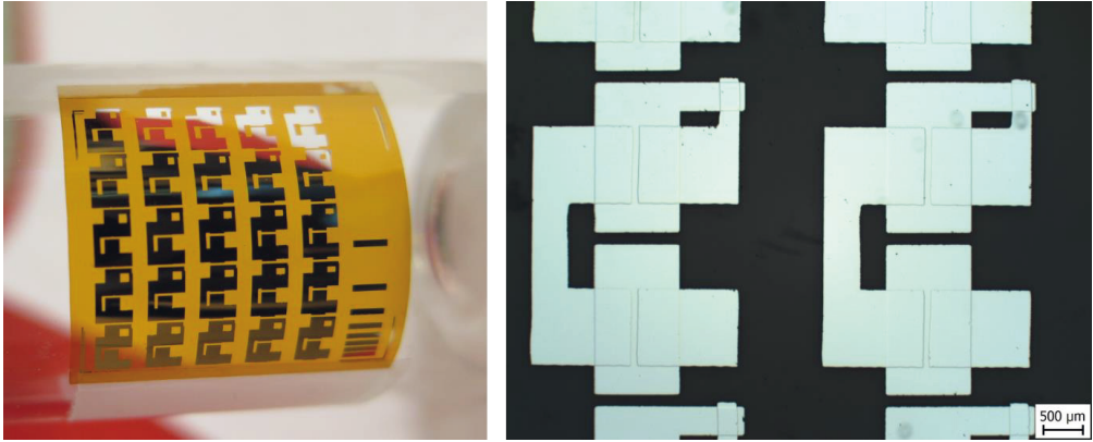
Figure 17. Figure Heading Flexible inverter circuit (a) A photograph and (b) optical micrograph. Scale bar 500 \mu\text{m} . (From Publication III) © [2021], Materials Science in Semiconductor Processing.
