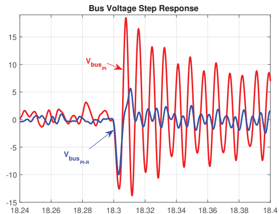
Fig. 9: The ac -coupled bus voltage response to a step change in the load VSI voltage.
