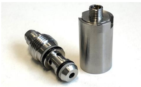
Fig. 8. Prototype on/off valve used in the study
