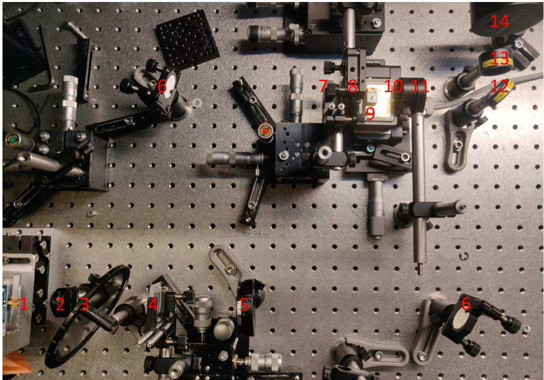
Figure 3.4. Second setup used in experiments with different lens configuration. 1. Assembly of figure 3.3 2. Isolator 3. Neutral density filter 4. Pre-focus lens 5. Waveplate 6. Mirrors 7. SA focusing lens 8. FA focusing lens 9. Nonlinear crystal 10. Crystal oven 11. Focusing lens for yellow light 12. Longpass dichroic mirror 13. Shortpass filter 14. Power meter
