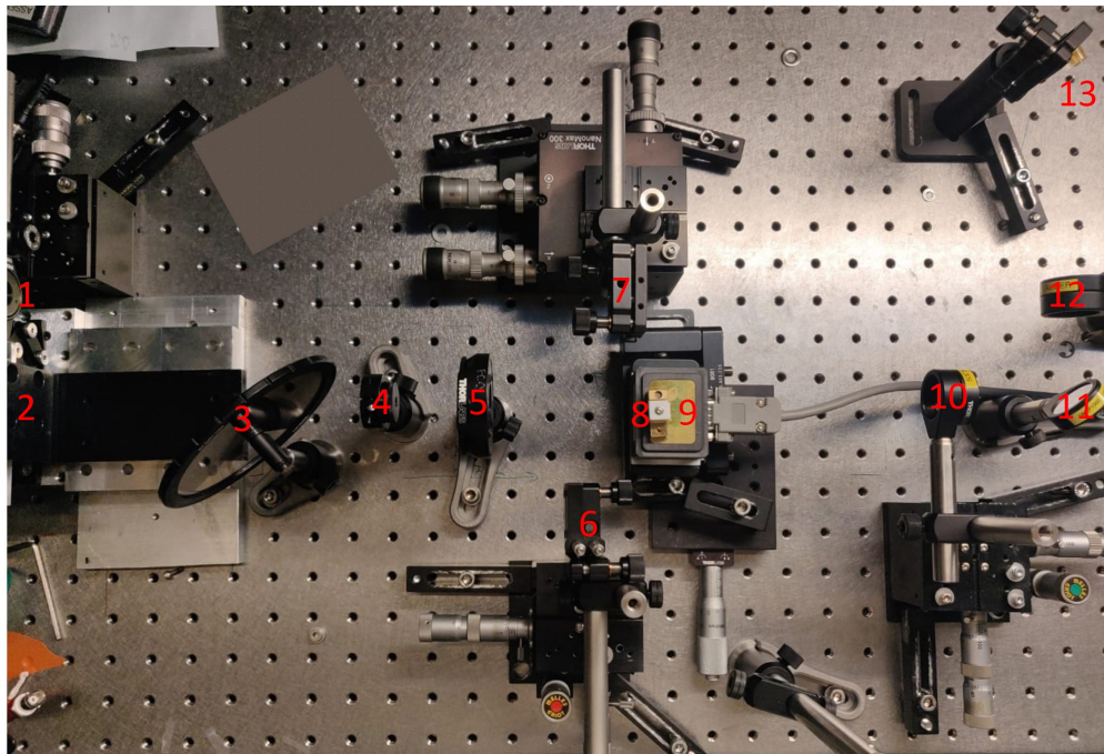
Figure 3.2. Setup used in experiments with RWG-DBR laser. 1. Collimation lens 2. RWG-DBR laser 3. Neutral density filter 4. Isolator 5. Wave plate 6. SA focusing lens 7. FA focusing lens 8. Nonlinear crystal 9. Crystal oven 10. Focusing lens for yellow light 11. Longpass dichroic mirror 12. Shortpass filter 13. Off picture is power meter.
