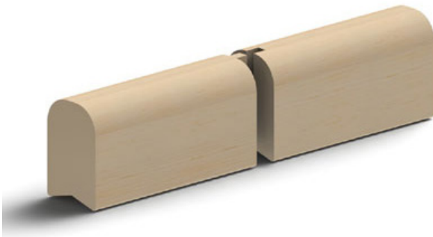
Figure 35 The continuation joint between logs
