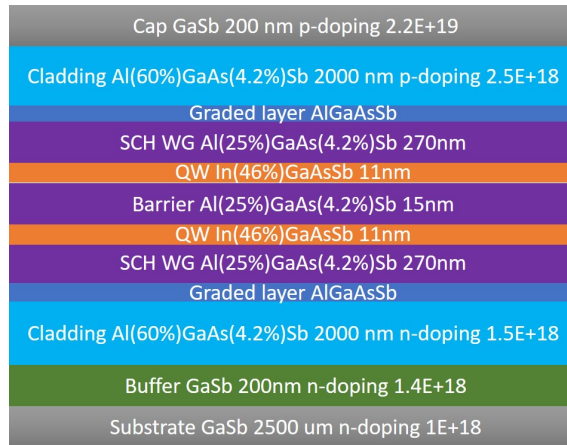
Figure 4.6. Epitaxial structure of 2.6 \mu\text{m} wavelength device
