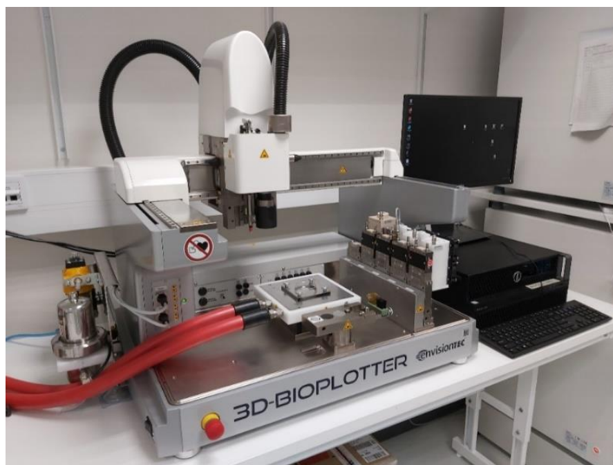
Figure 8. 3D-Bioplotter Manufacturer Series. The printing platform can be seen at the center of the device and the motor head with the camera and platform height control above it.
