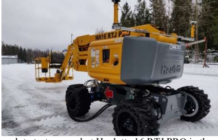
Fig. 1. Heavy-duty test-case robot Haulotte 16 RTJ PRO in the experimental environment.
