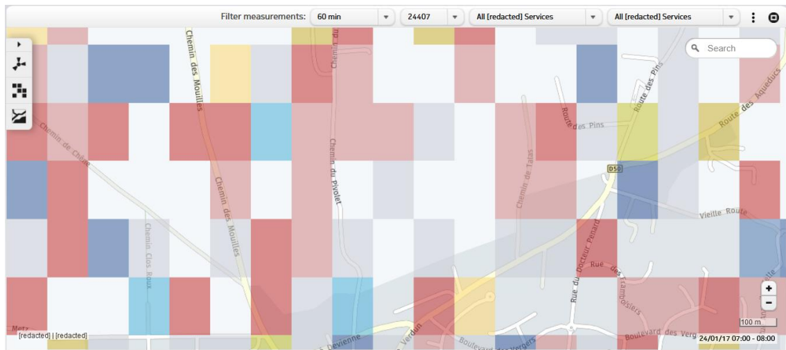
Figure 46. Geotiles shown with a guard value and a value-suppressing uncertainty palette applied. The red geotiles that fall below the guard value are given a less saturated color. Other geotiles that fall below the guard value are given a light grey hue.
