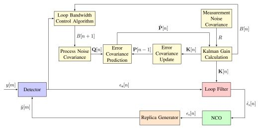
Fig. 4: Non-linear model of LBCA-based DSKF.
