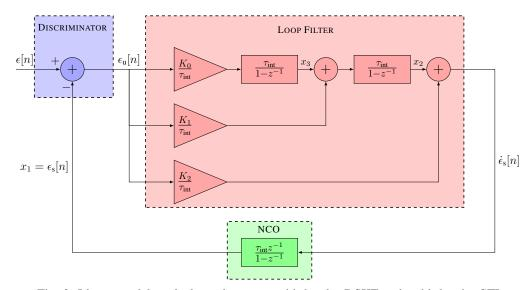
Fig. 2: Linear model equivalence between a third-order DSKF and a third-order STL.
