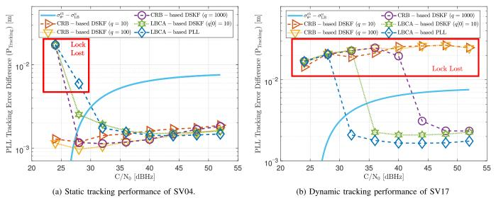
Fig. 5: Tracking performance of adaptive DSKF techniques in a third-order Costas PLL.
