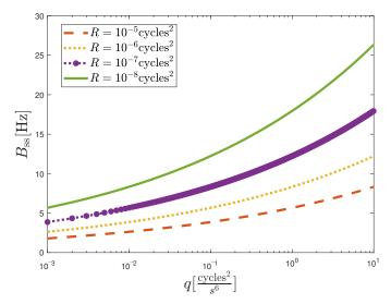
Fig. 3: Relation between steady-state loop bandwidth  $B_{ss}$  and process error variance q in a third-order DSKF.
