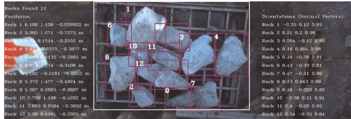
FIGURE 21 Real-time view of the rock detection scene. The positions and orientations for rock breaking are aligned to the left and right side accordingly [Color figure can be viewed at wileyonlinelibrary.com ]
