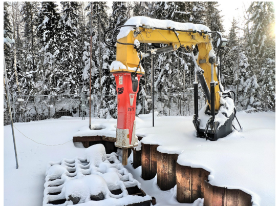
Fig. 1. RamBooms X88-540R breaker boom at the field test site at Tampere University.
