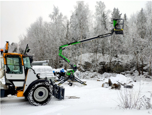
Fig. 7. Setup for experimental data gathering. The boulders are placed under the aerial work platform that is holding the TOF camera at a height of roughly 5 meters above ground.
