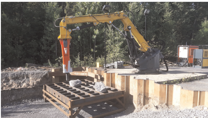
FIGURE 3 Rambooms X88-540R breaker boom at the field test site at Tampere University [Color figure can be viewed at wileyonlinelibrary.com ]
