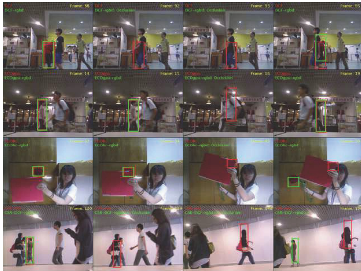
Fig. 4. Short-term and long-term occlusion examples comparing the original methods(red) and their RGBD versions(green). Top row – DCF, second row – ECOgpu, third row – ECOhc, bottom row – CSR-DCF.
