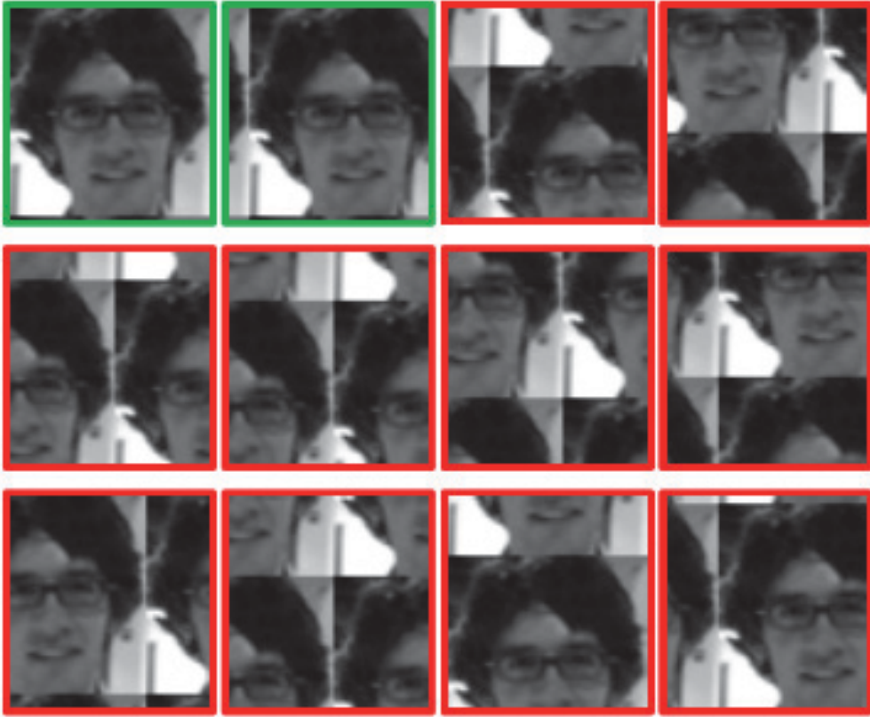
Figure 2.2 Boundary effects as a result of canonical correlation operation. Green boxes represent the positive and red boxes represent the negative implicit training samples respectively [40] ©2015 IEEE
