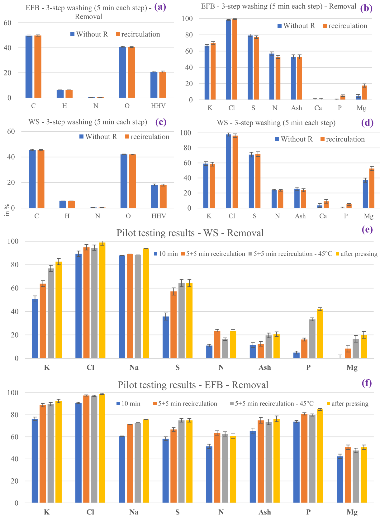
Fig. 3. Comparison between step washing with (SWWR) and without wastewater recirculation (SWFW) (a) and (b) for EFB; (c) and (d) for WS; (e) and (f) pilot testing results of SWWR.
