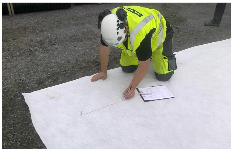
Figure 1. Sampling and marking of a geotextile on construction site
