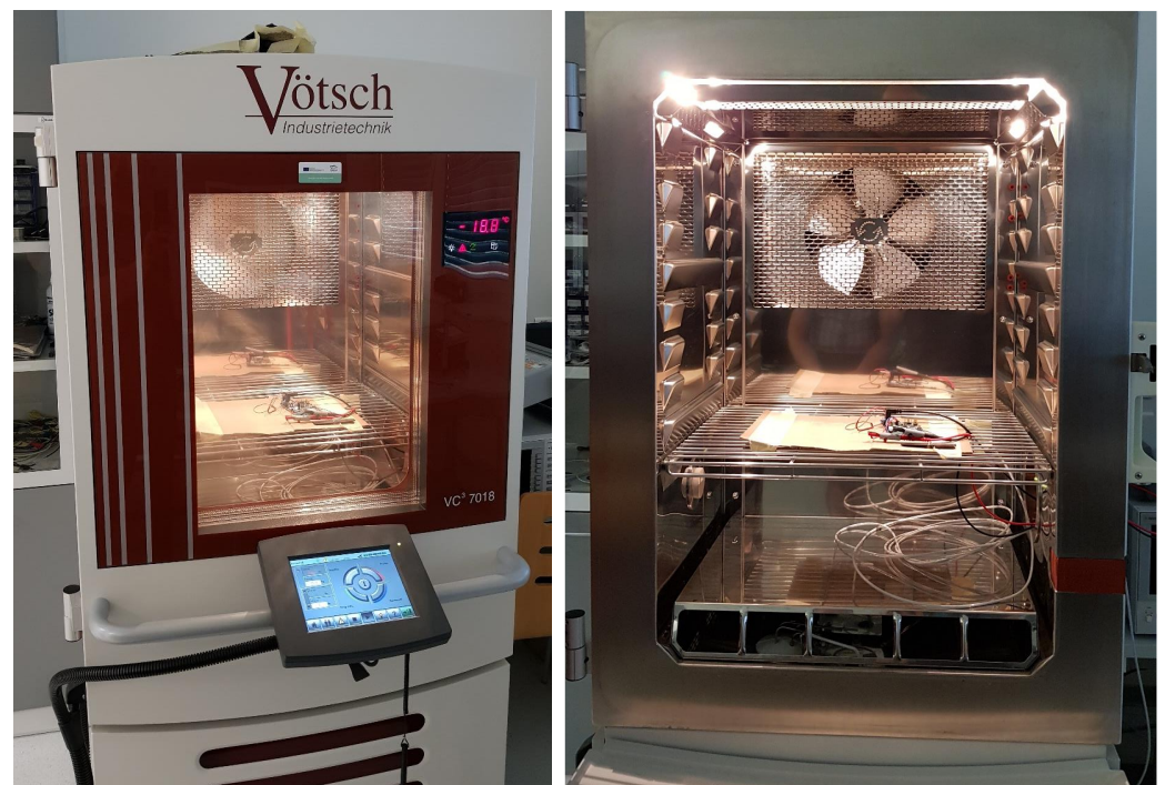
Figure 5. Durability measurements of devices in different climatic conditions in the temperature chamber Vötsch VC3 7018.
