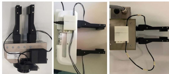
Fig. 3. Example of commercial grippers with integrated sensorized fingers: Schunk WSG-50 (left), Panda gripper (middle) and Schunk PG70 (right).
