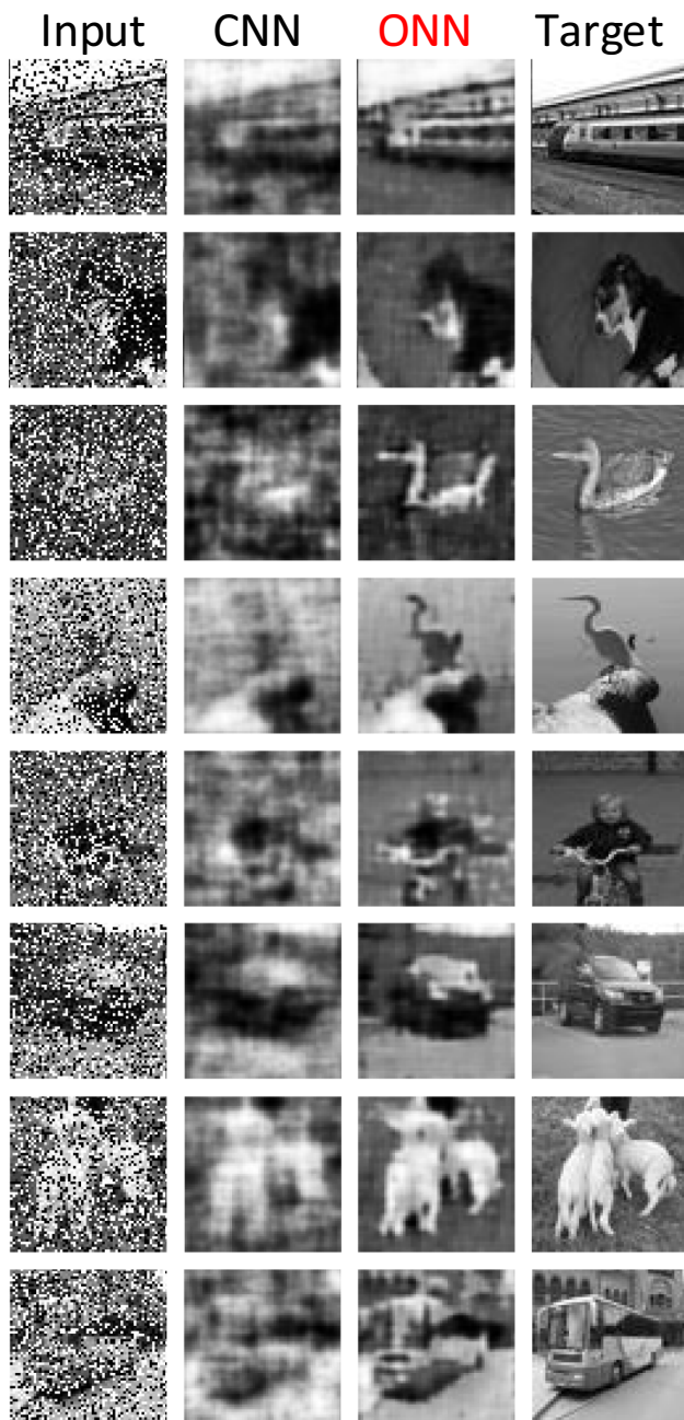
Fig. 9 Randomly selected original (target) and noisy (input) images and the corresponding outputs of the best CNNs and ONNs from the train partition
