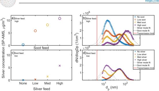
**Fig. 2.** Enhancement of elemental silver detection in the SP-AMS by the level of generated (a) soot and (c) silver and (b, d) corresponding particle size distributions from SMPS. Red line represents the vacuum aerodynamic diameter of 50 nm converted to electrical mobility, assuming the density of silver and spherical shape of particles.
