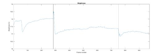
Figure 14: Brightness objective metric graph where the mobile phone first changes from the wide to the main and then back to the main
