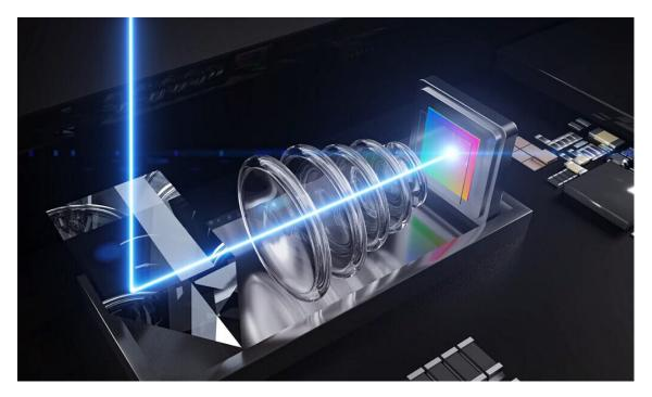
Figure 5: A periscope telephoto camera module [10]
