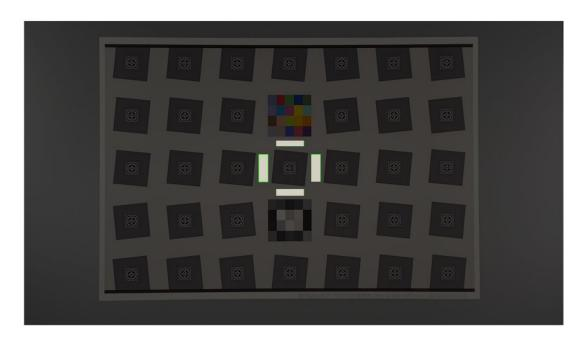
Figure 13: Gray patches detected in the SFRplus chart using object detection
