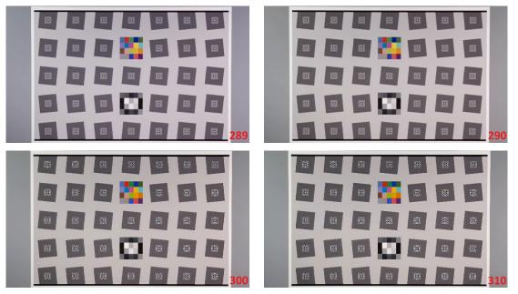
Figure 12: Some frames from a main to tele camera transition video. The numbers indicate the frame numbers. Frame 285 is using the main camera using the main and the rest of the frames are using the tele camera.
