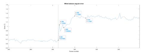
Figure 17: White balance graph for the first camera transition point
