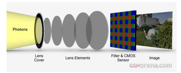
Figure 1: Components of an image sensor [3]
