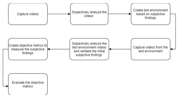
Figure 6: Zoom smoothness camera testing process
