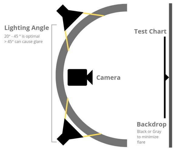
Figure 9: Test environment diagram [16]
