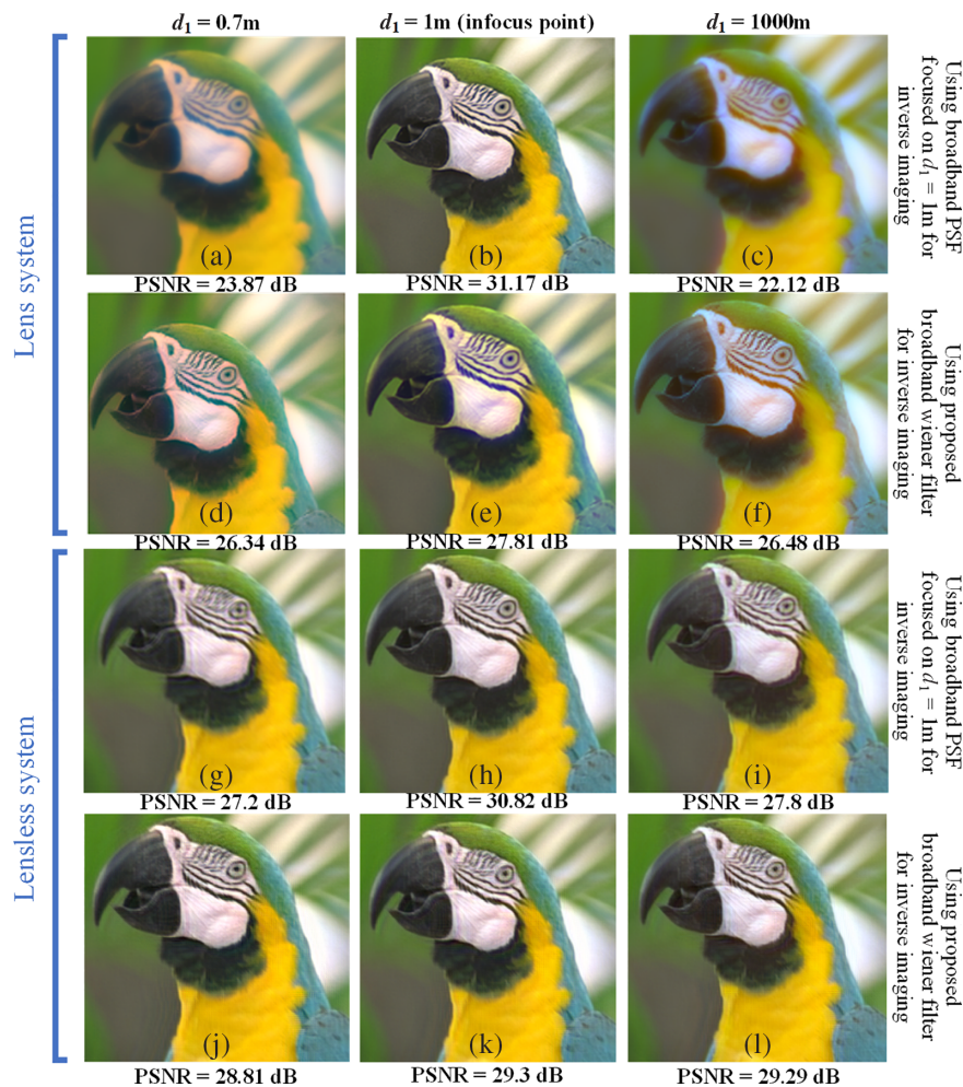
Fig. 5 Visual performance of the optimized lens and lensless optical setups with two different deblurring algorithms for comparison. The proposed BBWF [Eq. (13)] and Broadband PSF focused on d_1 = d_1^0 [BBFF, Eq. (14)] are exploited for both setups. The columns are given for different distances d_1 . The first two rows are for the system with the lens and the second pair of the rows for the lensless system. Comparing the results visually and by PSNRs, we may conclude that the best result is given by the lens system for the focal distance d_1 = 1 . However, for defocus situations, the performance of the lensless system is advanced. Overall, the comparison corresponds to the conclusion following from the analysis of PSNRs in Fig. 4, the best performance is achieved by the proposed MPM system with the Wiener inverse filtering (BBWF): the last row of the table.
