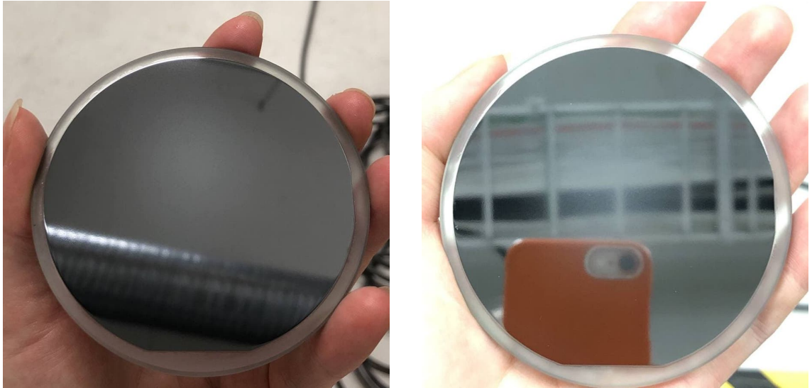
Figure 5.8. GaAs wafer surface after 30 min of polishing with OCON-353 pad.
