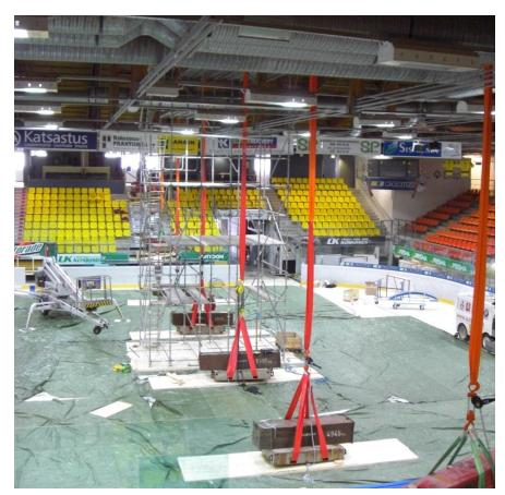
Figure 2. View of the test loading, with weights on the floor lifted up.
