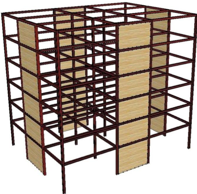
Figure 16. The principle of the steel moment frames with CLT infill panels (Bezabeh and Tesfamariam 2016).
