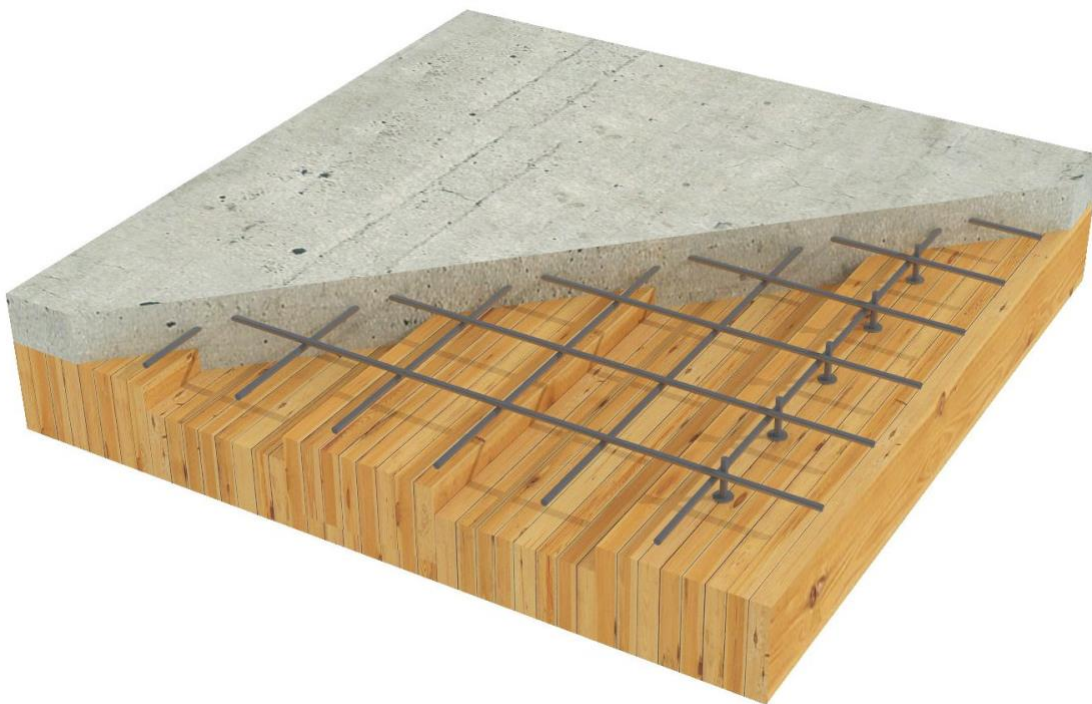
Figure 19. Visualization of the timber-concrete composite floor (©StructureCraft).
