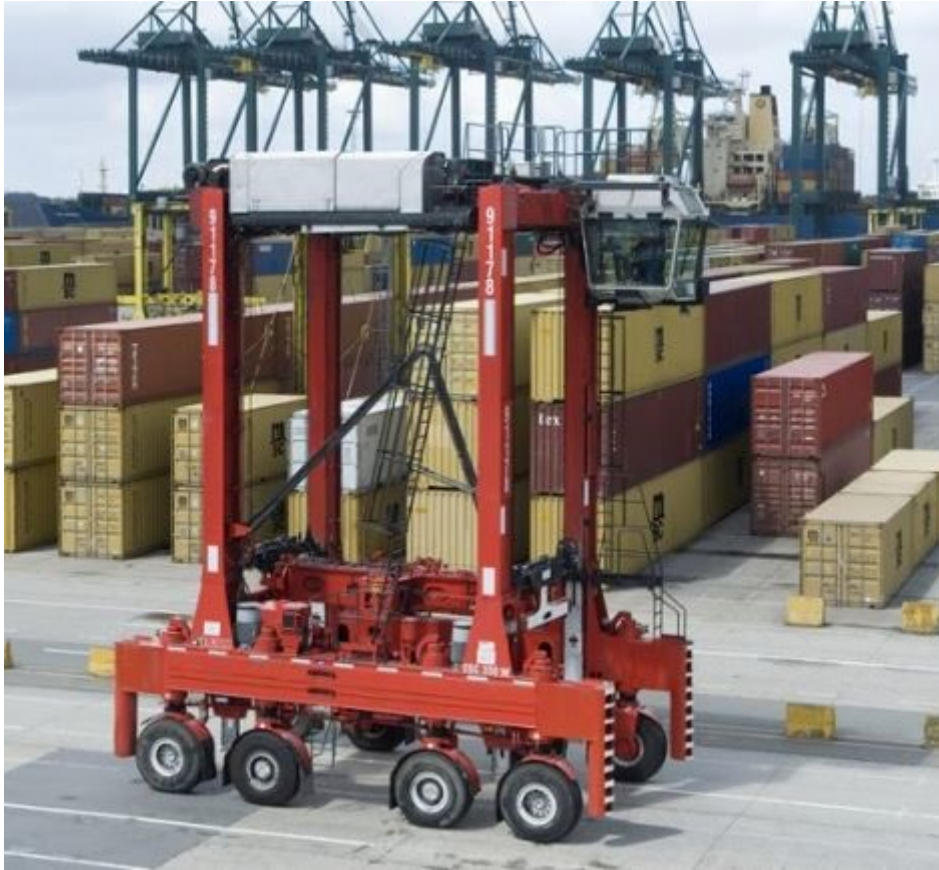
Figure 3. A straddle carrier. Adapted from [14].
