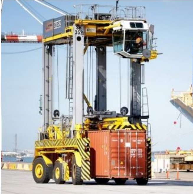
Figure 4. Shuttle carrier transporting a container. [13]
