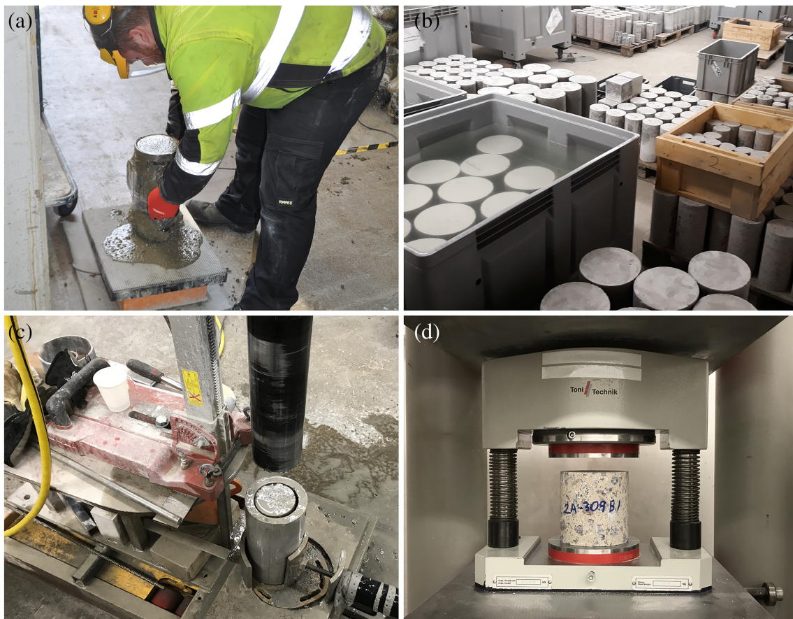
FIGURE 4 The different stages of the experimental programme: compaction (a), storing (b), drilling (c) and testing (d)
