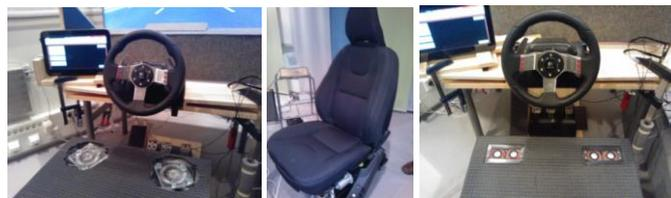
Fig. 1. The Haptic Seat uses a pair of rotatory motors (left) and TEAX25C10-8/HS actuators (right) to generate feedback.
