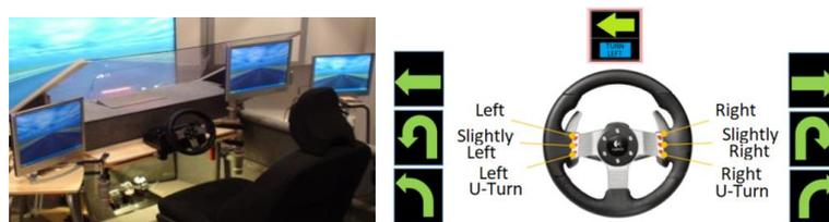
Fig. 2. Lab setup and data collected while drivers performed the LCT (primary) and Navigational (secondary) tasks.
