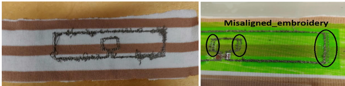
Figure 5. Encountered embroidery challenges: Thread clusters (left) and misaligned embroidery rounds (right).
