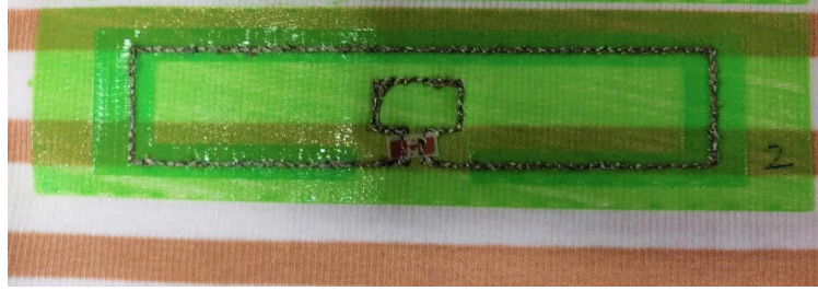
Figure 3. Embroidered antenna pattern and attached IC component on a 3D-printed structure.
