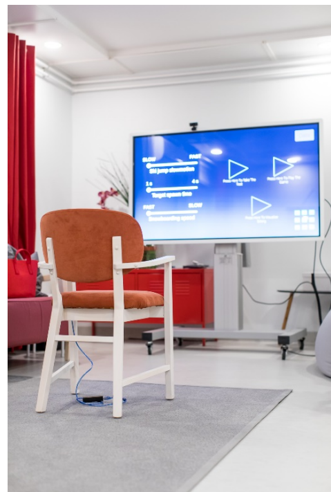
Fig. 2. The game set-up consisted of the smart gaming chair and the big touch screen (starting menu on screen).
