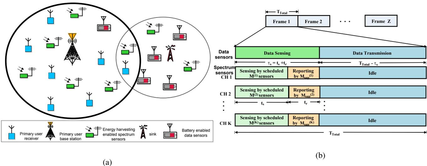
Figure 1: (a) System model of the considered HCRN; (b) Frame structure of the SSR-based HCRN.
