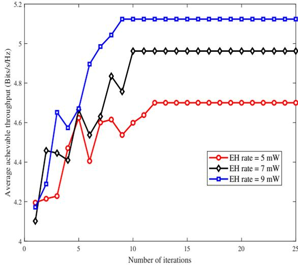
Figure 3: Average achievable throughput vs. number of iterations for different EH rates.
