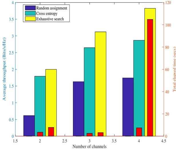
Figure 2: Comparison of throughput for SSR scheme with CE algorithm, random assignment and exhaustive search methods.
