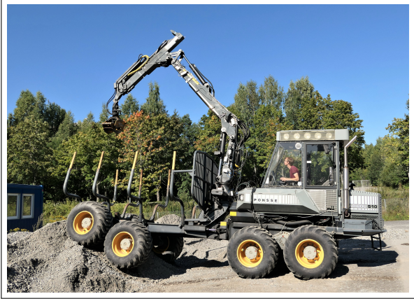
Fig. 3. The forest forwarder that acts as our mobile test platform, complete with manipulator arm.
