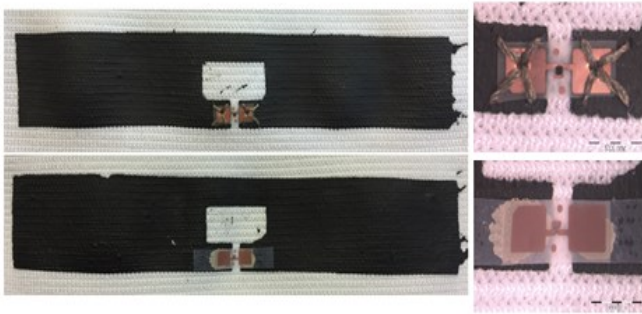
Fig. 2. Ready RFID tags: Embroidered (top) and epoxy-glued (bottom) interconnections.
