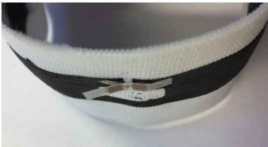
Fig. 5. Broken epoxy-glued antenna-microchip interconnection.
