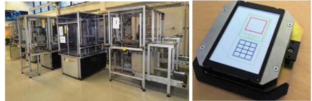
Figure 4. FASTory Assembly Line and the final product on a pallet
