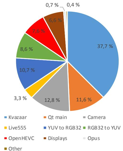
Figure 8. Relative CPU usage with 720p resolution and QP 27.
