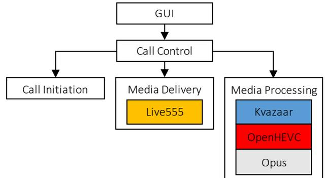
Figure 1. High-level architecture of Kvazzup.
