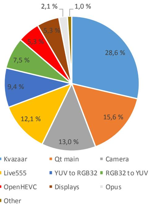
Figure 7. Relative CPU usage with VGA resolution and QP 32.
