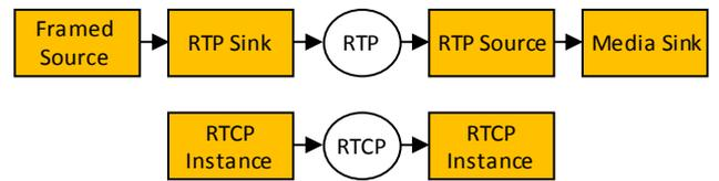
Figure 4. RTP/RTCP delivery flow with Live555.
