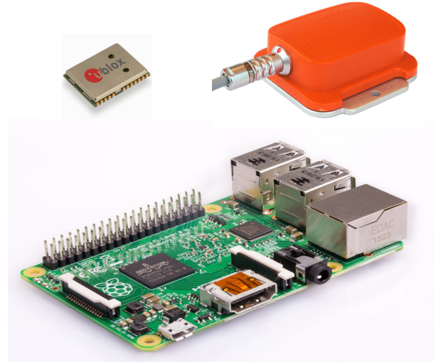
Figure 2: The data logger comprising a Raspberry Pi-2B board, u-blox GNSS receiver and an Xsens IMU.
