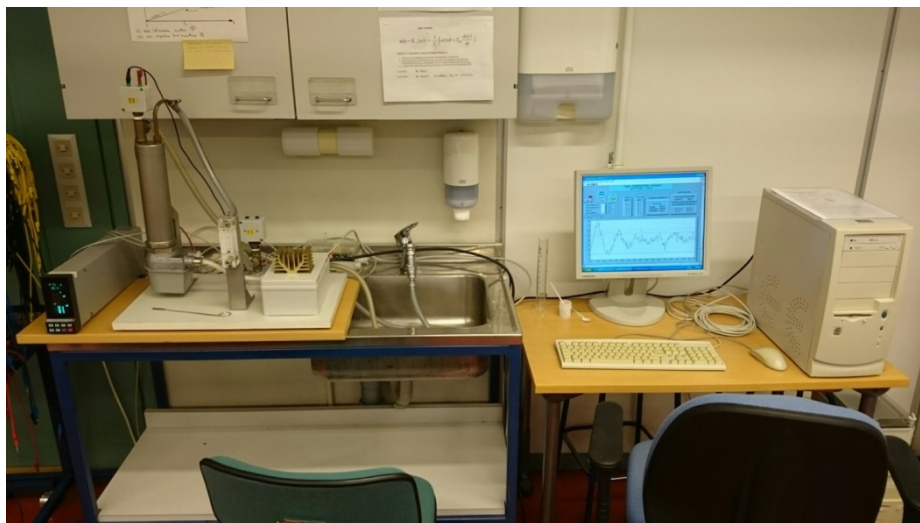
Fig. 1. Water heating system (left) and process monitoring computer (right).
