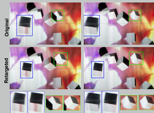
Figure 2: Retargeting results recorded after displaying on a light field display. Top row: two views of original light field content. Middle row: corresponding depth retargeted views. Bottom row: close-ups of retargeting results.
