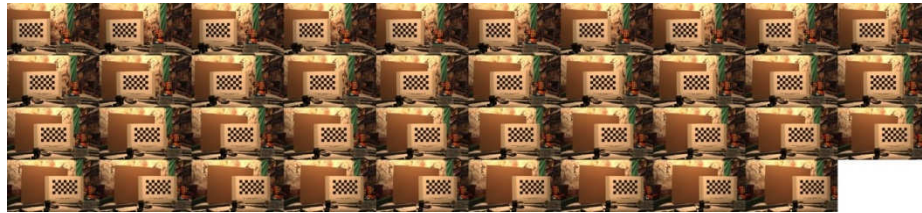
Fig. 5. Example of views taken with 11mm distance using LPS. Original data contain 400 views of size 1980x1080px taken with 1mm distance.
