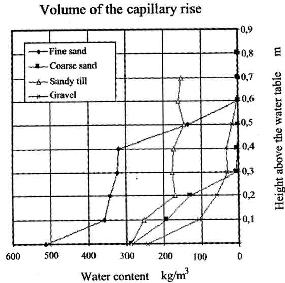
**Figure 5** Vertical capillary moisture equilibrium curve of different coarse-grained soil types typically used as a drainage layer in Finland.
