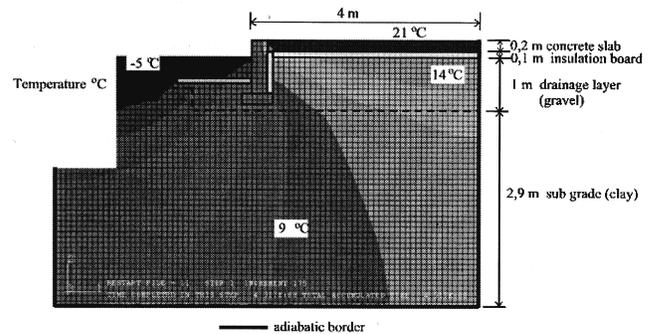
**Figure 3** The prevailing temperature field at the subgrade and ground floor structures after 15 years of thermal load caused by heated building.
