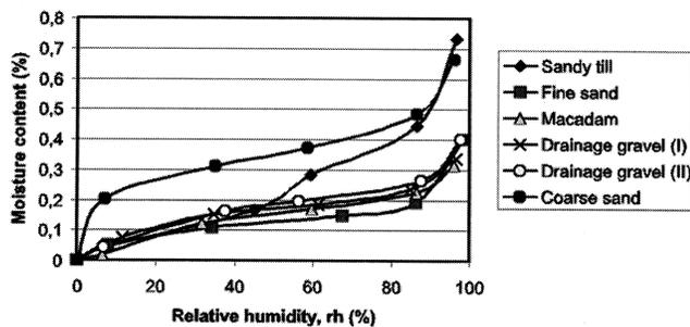
**Figure 1** Hygroscopic equilibrium moisture curve (absorption) of different coarse-grained soil types typically used as a drainage layer in Finland.
