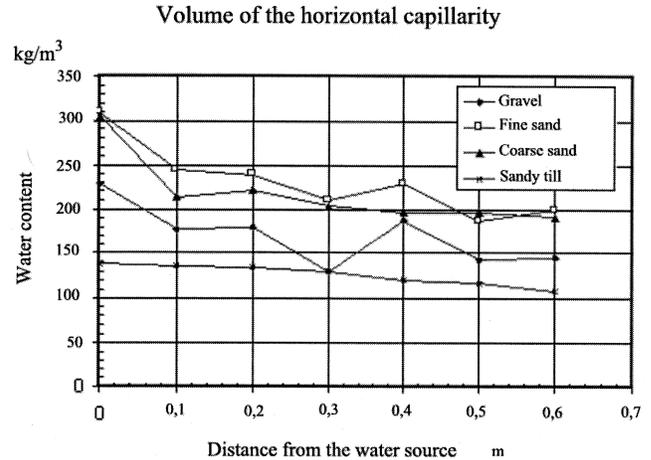
**Figure 6** Horizontal capillary moisture flow curve of different coarse-grained soil types typically used as a drainage layer in Finland.
