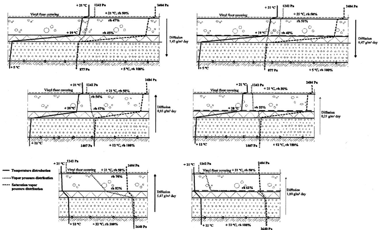
Figure 4 Temperature, saturation vapor pressure, and vapor pressure distributions of a ground slab with and without vapor retarder beneath the insulation in different subgrade temperatures.
