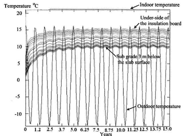
**Figure 2** Observed temperature changes at the subgrade and ground floor structures at the numerical finite element modeling (FEM).
