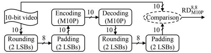
(b)  $M10P_{8,8}$ : the M10P encoder with 8-bit input and 8-bit output.
