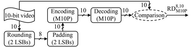
(c)  $M10P_{8,10}$ : the M10P encoder with 8-bit input and 10-bit output.
