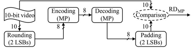
(a) MP: the MP encoder with 8-bit input and 8-bit output.
