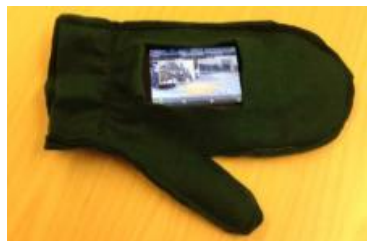
Figure 5. SeekThrough prototype: a smart phone attached to a self-made glove.
